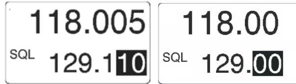
8.33 kHz channel spacing (left) / 25 kHz channel spacing (right)
